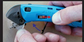
Insert new blade onto blade retainer by aligning blade notch with alignment tab. Close Blade Lock. Pull blade change button back to the locked position.
