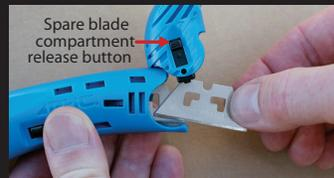
Unlock spare blade compartment by pulling back on the release button. Rotate compartment upward and safely pull spare blade out. Close spare blade compartment.
