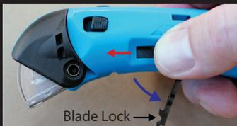
Disengage blade lock. Push blade change buttons forward in tandem on both sides of the safety cutter.
