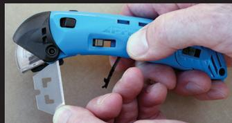
Remove used blade from blade retainer and dispose of safely.
